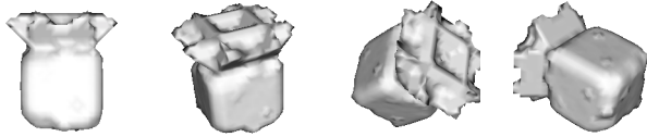
Figure 8: Stereo-based reconstruction of the scene in figure 7: convergence is achieved everywhere but on the white face of the cube.
