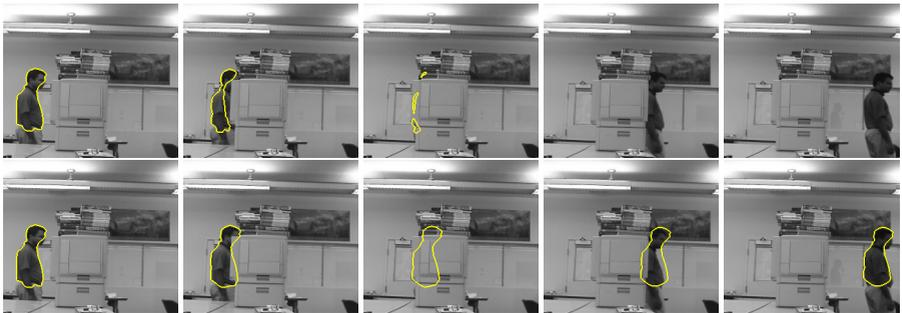
**Fig. 2.** Tracking a man through an occlusion. Bottom row shows the results of using a prediction (filtering) on the centroid and the isoperimetric ratio, and then penalizing deviations of the contour away from predicted parameters by (13) ( $\alpha = 50000$ ,  $\beta = 100$ ). The top row gives the result with no such penalty. Both use Sobolev active contours.
