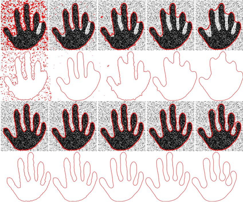
**Fig. 1.**  $\mathbb{L}^2$  regularization (top two rows). Left to right:  $\alpha = 1000$ ,  $\alpha = 1000$  followed by curvature smoothing to remove the noise (least number of iterations to remove noise),  $\alpha = 10000$ ,  $50000$ ,  $90000$ . The image-based term is Chan-Vese. Sobolev elastic regularization (bottom two rows). Left to right:  $\alpha = 0, 0.1, 5, 10, 25$ . The second and fourth row show the same result as the row above them, but the image is removed for visibility.
